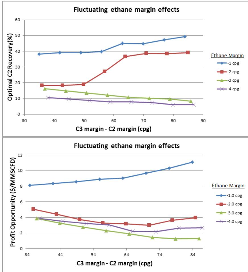
Figure 6 – Optimal response to ethane margin fluctuations
